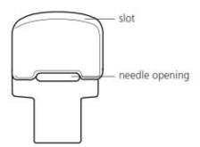
The slot in the foot is used to gather a ruffle and stitch it to a flat piece of fabric all in one operation. The fabric to be gathered is fed under the foot and the flat piece of fabric is fed into the slot, keeping it from touching the feed dog.
